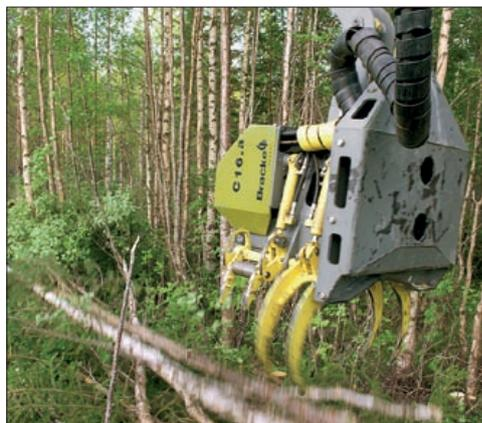
In its tilted position, the C16.a can be used as a grapple for loading and unloading.
